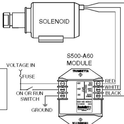
3. **S500-A5 & A50 Modules** - After making the final wiring check, energize the solenoid hold coil by turning the switch to the [on] position and manually push the solenoid plunger to the seated position. The plunger should remain seated.
