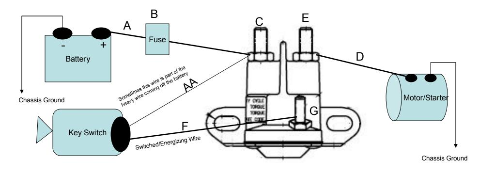
Note: Do not remove nut from stud (C) or stud (E). Do not remove nut from stud (G)
